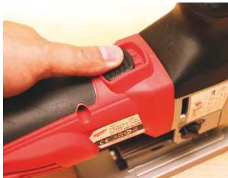
▲ A top-mounted power slider is easily accessible for left- or right-hand operation
